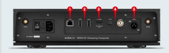
Ethernet port for wired network connection
